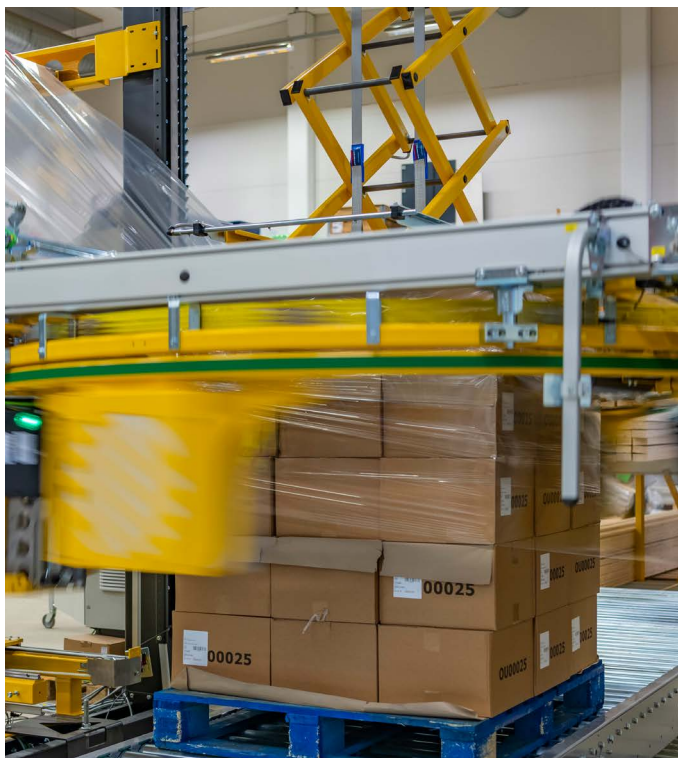
Real time data collection, on pallet during wrapping cycle
